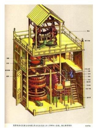
The world's first mechanical clock -Water-driven Spherical Birds – was invented by Yi Xing, a Buddhist monk in 725 A.D.. It was operated by dripping water which powered a wheel that made one revolution in 24 hours. Hundreds of years later, the inventor Su Song developed a more sophisticated clock called the Cosmic Empire in 1092, 200 years earlier before the mechanical clock was created in Europe.
